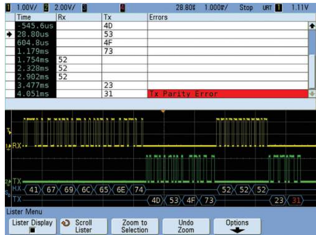
Figure 2. InfiniiVision Series scopes provide flexible RS-232/UART decoding formats including binary, hex, and ASCII.
