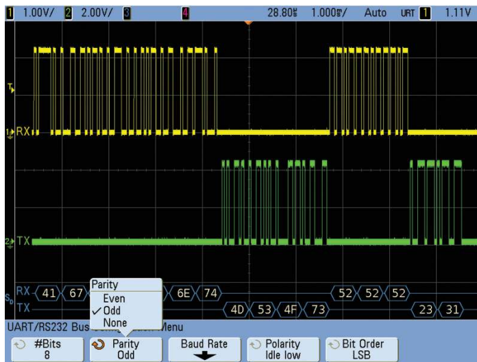
Figure 1. Defining the RS232/UART protocol structure
